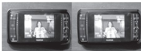
Back view of the Fujifilm Real3D Finepix Digital 3-D W1 camera showing the 3D lenticular preview and playback screen – photo by David Starkman
