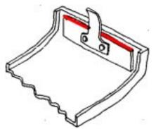
Fig. 2—Location for gasket on the camera door.
