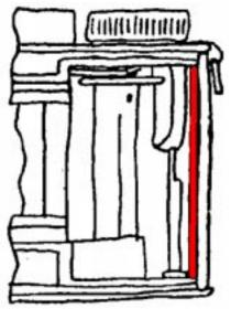
Fig. 3—Location for gasket on the camera body.
