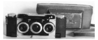
chip (24x36mm) in the 35mm film camera that you now shoot with. This will yield up to 29 stereo pairs in a 36 exposure roll of film! This is by far the most popular and widely supported form of 3D photography today, and has been since it took off in the 1950s. It is the most highly recommended format to start out with!
